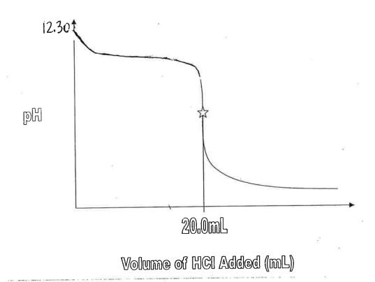
A 30.0mL sample of the base  $B^{\text{-}}$  was titrated with 0.200M HCl, and the titration curve above was obtained. Calculate the  $K_b$  of  $B^{\text{-}}$  .
