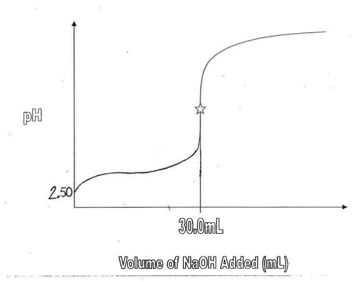
A 32.0mL sample of HA was titrated with 0.20M NaOH, and the titration curve shown was obtained. Calculate the K<sub>a</sub> of HA.
