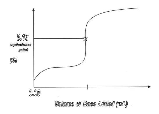
Though two parts of this curve are different than the strong acid/strong base curve, the sharp vertical rise is still present.
