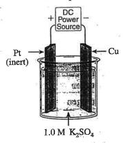
33. What is the equation for the anode reaction?
